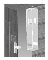
4. Attach door keeper and emergency key plates to hoistway door.
