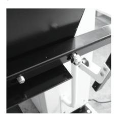
The ramp roller should align and make contact with the ramp roller guide.
