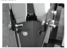
**Step 4:** Attach the ramp roller arm by bolting it to the underside of the ramp.
