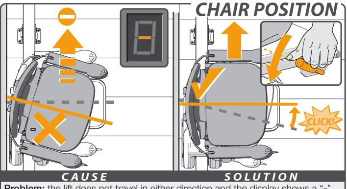
Problem: the lift does not travel in either direction and the display shows a "-".Cause: the seat is not locked and is in a swivelled position.Solution: swivel the seat using the handle located to the left or right under the seat, until it "clicks" into position.
