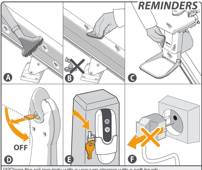
[A]Clean the rail regularly with a vacuum cleaner with a soft brush. [B]Any dirt on the rail can easily be removed with a slightly damp cloth. Under no circumstances should you use cleaning product when cleaning the rail. [C]Clean the stairlift regularly with a damp cloth.
