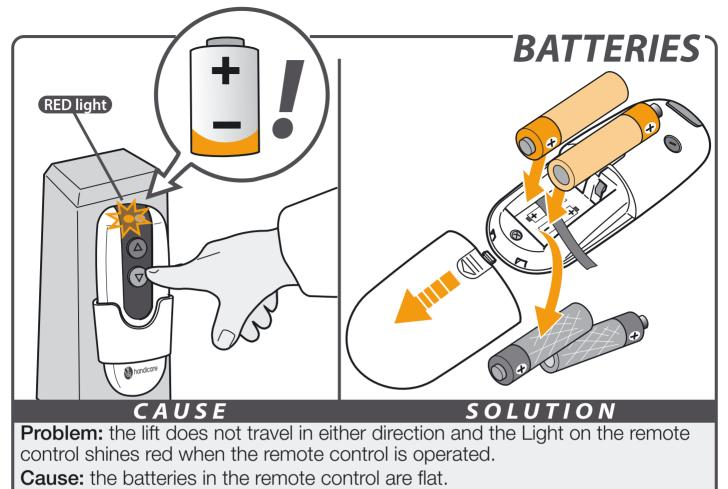
Solution: replace the batteries in the remote control.
