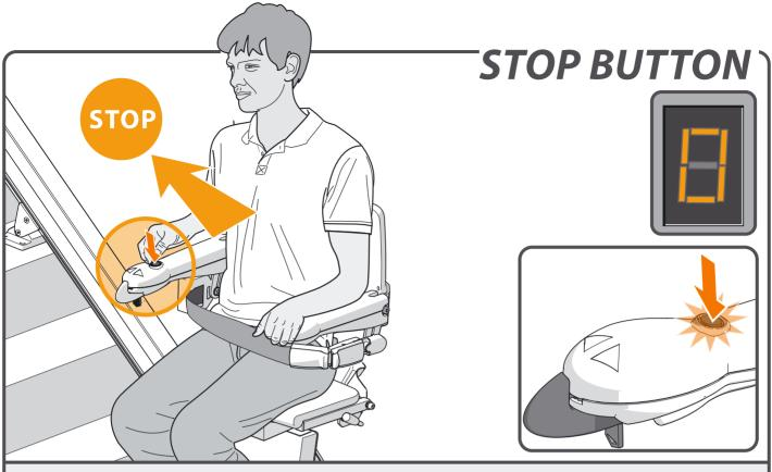
In an emergency, press the stop button once. The lift stops straight away. To release the lift, press the stop button again.
