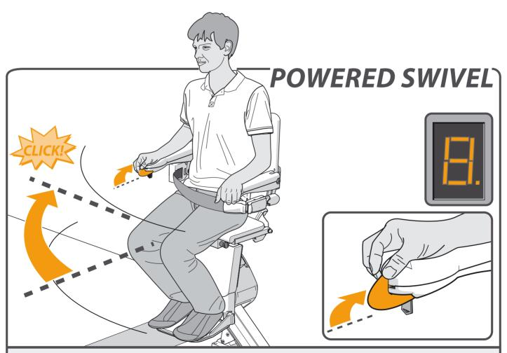
The POWERED SWIVEL SEAT option let you swivel the seat automatically to face the direction you are going to walk. To do this, push and hold the joystick in the direction of travel.
