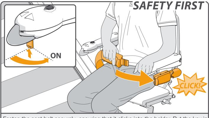
Fasten the seat belt securely, ensuring that it clicks into the holder. Put the key in the switch and turn it ninety degrees clockwise. Check that the chair is in the locked position.
