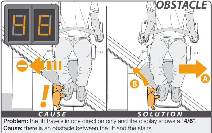
Solution: move the lift in the opposite direction {A} and remove the obstacle {B}.
