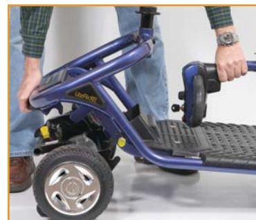
While squeezing the release lever, pull up on the rear frame
