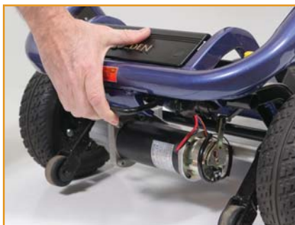
To separate the rear transaxle from the frame, squeeze the release lever located on the underside of the frame
