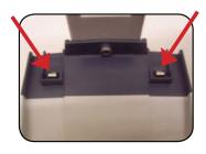
Make sure the contact points of the control box and the battery are not damaged or corroded. If there is corrosion clean with Scotch-Brite™ pad. Put some dielectric grease on the contact points before reattaching the battery.
