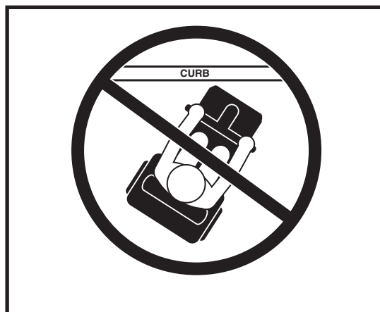
Figure 7. Incorrect Curb Approach
