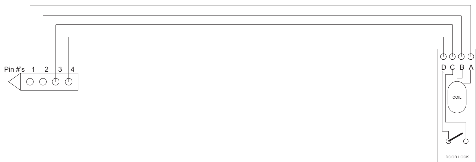
Typical Hall Call Station Diagram { } Indicate Pin Number
