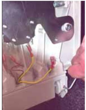
Tap mounting bar through bracket and remove footrest assembly, pull loom out of footrest, one connector at a time, remove 3 bolts and reposition bracket. Replace bolts and feed loom back through hole 1 connector at a time. Reattach to chassis leg by knocking mounting bar back through bracket – be careful not to damage footrest limit loom. Tighten grub screw and reattach lever link bracket with 2 screws. Rehook leverlink footrest spring.
