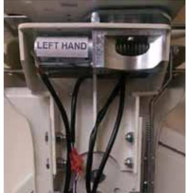
If the stairlift has a powered swivel, connect the swivel motor loom (Red & Black). Black - Black, Red - Red for a Right hand Lift, Black - Red, Red - Black for a Left Hand Lift. Connect swivel limit loom as shown in pictures, Purple - Purple, White - White for Both Hand Lifts. Finally pass chair & display loom up through centre of swivel boss.
