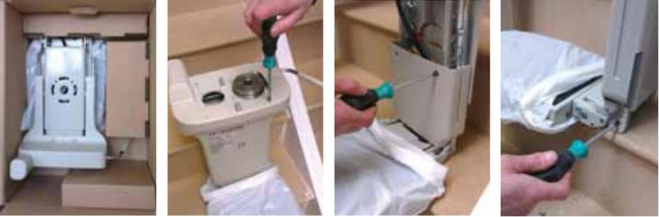
Attach Chassis Leg to Drive Unit ensuring all cables pass through central hole correctly.
