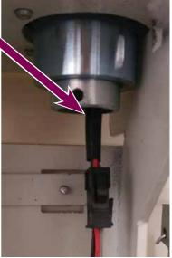
Fit Grey ribbon display loom & 2 x IR receiver looms on to chassis leg upper cover. Temporarily leave on footrest.
