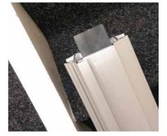
Slide bottom Jointing Plate into lower section of track and tighten one bolt to hold in position. Place lower section of rail onto the staircase and slide top section into position until the gap closes completely. Loosen bolt on bottom Jointing Plate and slide back up until it straddles track joint. Tighten all 8 bolts.
