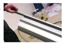
Upack Drive Unit. Load at top of track carefully. Ensure that lower carriage rollers are located into rail extrusion channels correctly and that drive and OSG pinions do not catch. Lower Drive Unit, slowly down the Rail Extrusion until drive pinion rests against lower rack section. Do not install top section of gear rail until carriage is loaded on rail.
