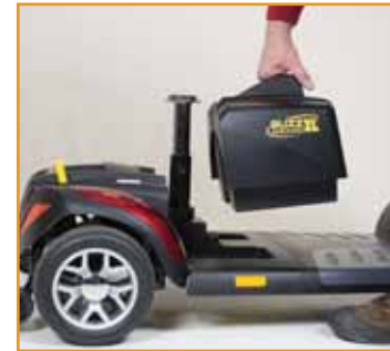
Step 2: Pull out the battery pack!
